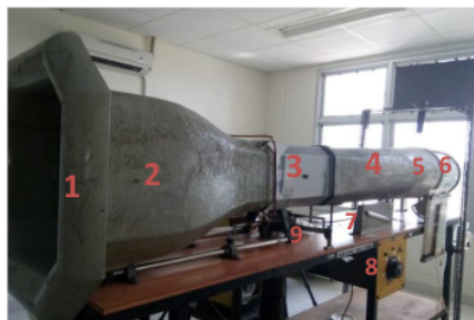
Figure 2 Wind tunnel used in the research with its elements [10]
